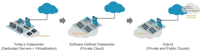
Figure 1-1: Data centers are evolving to include a mix of hardware and cloud computing technologies.
