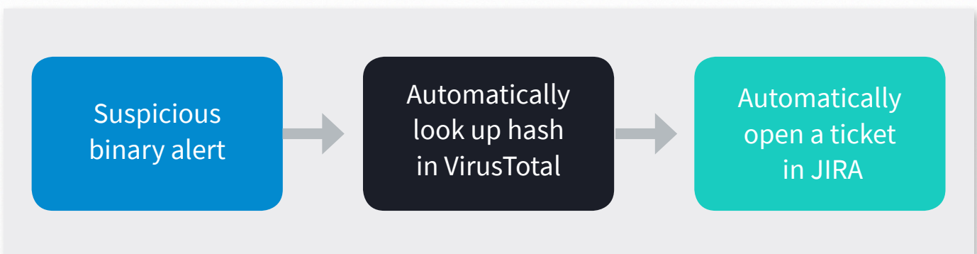
Figure 4 – Sample workflow of automation of two manual incident response processes.
